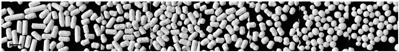
Fig. 6. Images of MCCII particles after varied spheronization times (10, 20, 30, 45, 60, 120, 240, 480 s), scale \hat{=} 2.0 mm.
